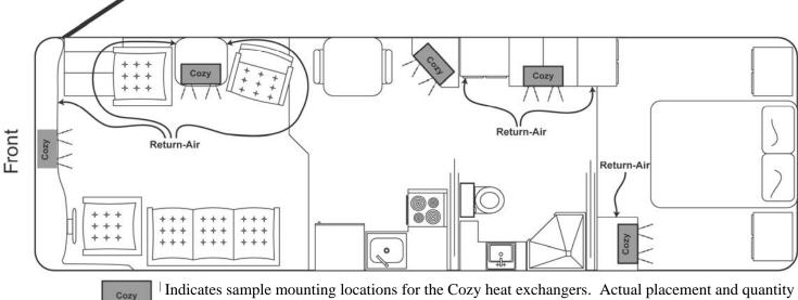
Cozy Indicates sample mounting locations for the Cozy heat exchangers. Actual placement and quantity vary based on the individual design of the coach. For specific design assistance, contact Aqua-Hot at 303-659-8221
