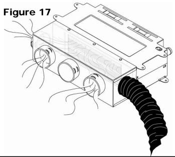
smaller vent as seen in Figure 18. The plenum allows only the desired outlets to be opened by removing the metal insert on the vent.
