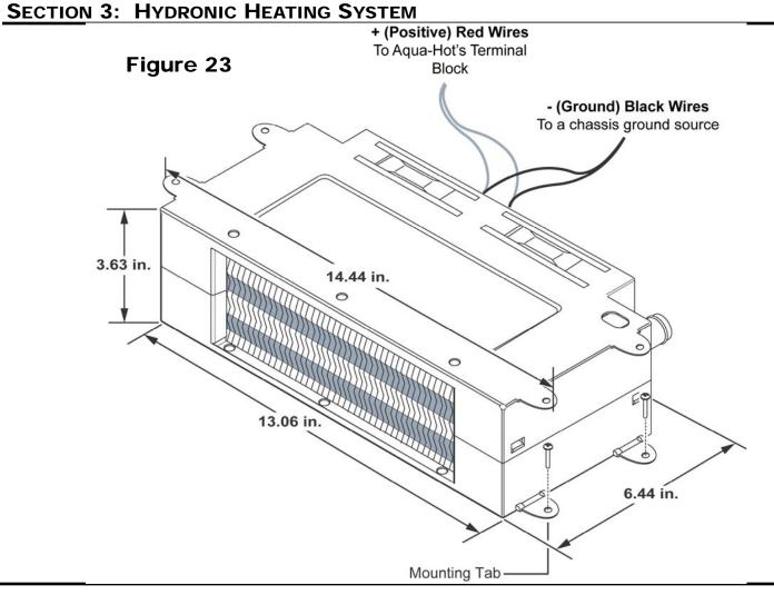
When wiring the heat exchangers in-parallel, the main 18gauge wire is split to allow the heat exchanger wires to combine with the main wire to be powered or grounded, respectively.
