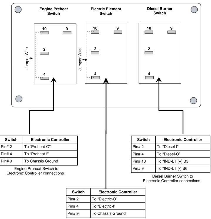
Electric Element Switch to Electronic Controller connections
