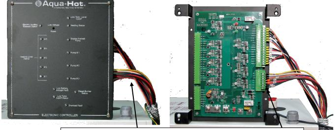
Connect corresponding 9 and 16 pin connectors from wiring harness
